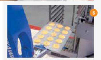
The tray is being replaced in the right position in the rack
