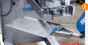
The tray is placed in the right position underneath the depositing heads
